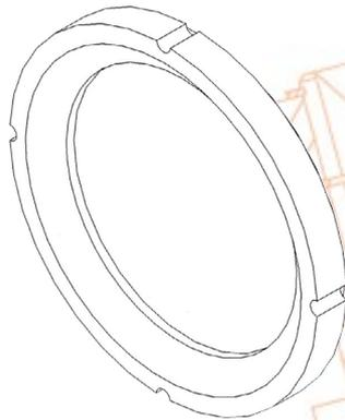
Specially designed APV seats allow equalisation of pressure in the ball cavity which reduces operating torque and increases seat life.
